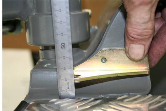
1. With appropriate bracket (see picture) match curve on bracket with bar side plate until a height of 15mm is reached from the underside of strut bracket, to the top of the chequer plate. Drill holes and rivet bracket to the side plate.
