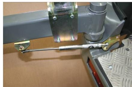
Note: With this bracket clamped into position, a measurement of 275mm should be achieved between the two hole centres of each bracket.
